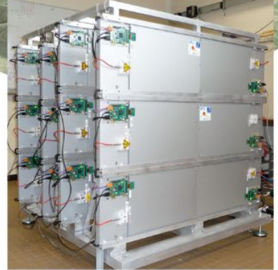
4 layers of gas resistive plate chambers (GRPCs)
