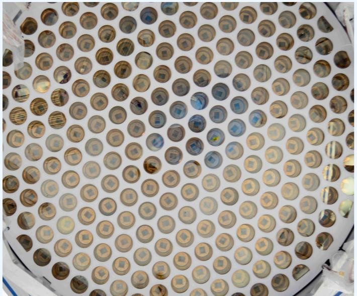
PMT array (494 PMTs in total,
