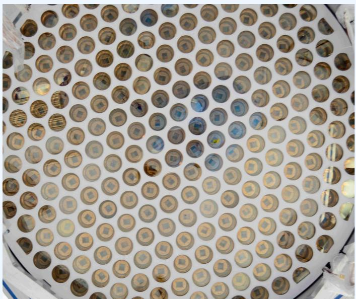
PMT array (494 PMTs in total,
