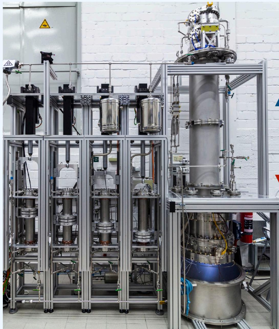
**Constant removal of emanating radon from xenon using difference in vapor pressure**
