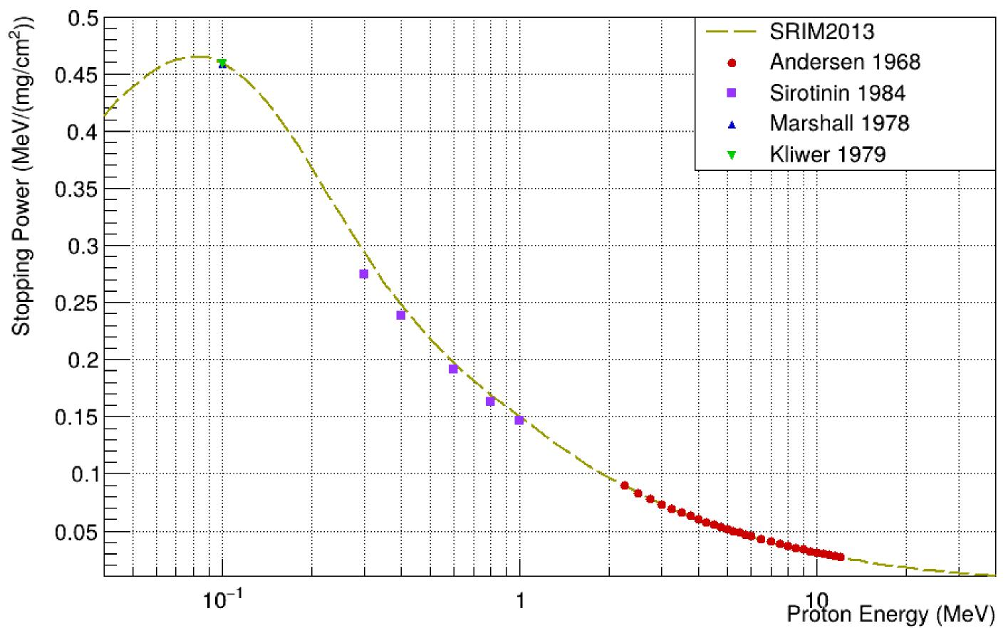
Target thickness can be estimated from SRIM stopping powers by integrating energy loss of protons in scandium. The calculation links the required  $\Delta E$  to an equivalent material depth ( $\rho_{Sc}=2.99~{\rm g/cm^2}$ ).
