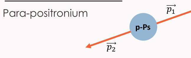
Isotropic decay into 2 back-to-back photons with energies of 511 keV
