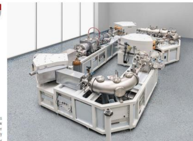
IonPlus manufactured Accelerator Mass Spectrometer. Pictured is the Multi-Isotope Low Energy AMS (MILEA) to be used at the Lancaster University based facility © IonPlus
