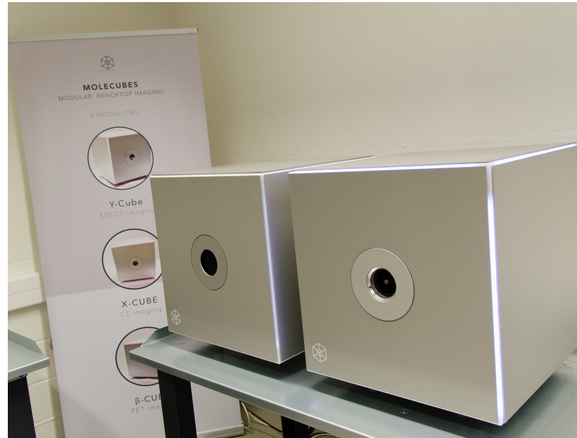
2017 Molecubes Beta + X Cube 8 mm thick LYSO 13 cm axial FOV still sub mm
