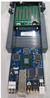
Fig. 8: FTAB with amplification stage (not visible) and power supplies (green board)
